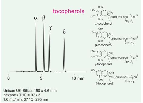
The Unison series of columns provides authoratative results in normal phase separation using its silica stationary phase. This high level of performance is in addition to its extraordinary resolution, higher than conventional 5um columns.
