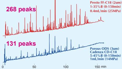
Presto FF-C18 enables unbelievable separation power for peptide mapping. Accurate trace analysis for peptides is very important for proteome analysis, but can be compromised with porous ODS column - due to adsorption in micro-pores.
