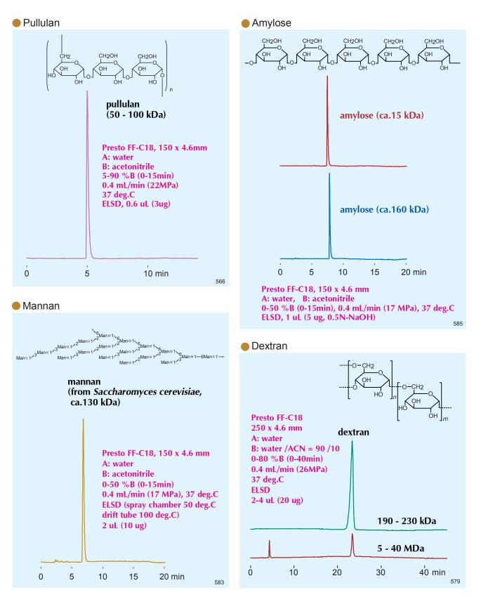
Reversed-phase separation for non-ionic polysaccharides on Presto FF-C18 does not require any pH modifier. Excellent peak shape was observed for several non-ionic polysaccharides using water / acetonitrile gradients. Polysaccharides contain multiple OH groups, and different concentrations of acetonitrile may be required for proper elution. The data shows that retention will be similar for homo polysaccharides larger than 10kDa. Peak shape is dependent upon molecular size distribution.
