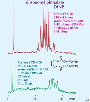
On conventional porous ODS, Phthalic di-ester has numerous branched-chains with the same MW that co-elute. In contrast, Presto FF-C18, at a low flow rate, recognizes the alkyl chain isomers and is more sensitive. When mobile phase composition and flow rate is optimized, Presto FF-C18 can at times achieve amazing peak shape for small molecules.
