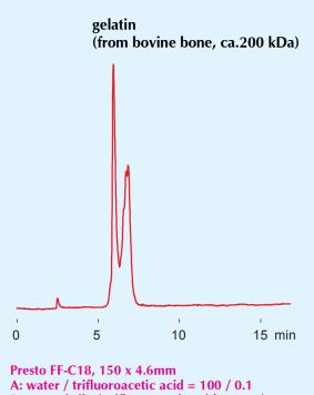
A: water / trifluoroacetic acid = 100 / 0.1 B: acetonitrile / trifluoroacetic acid = 100 / 0.1 10-90 %B (0-15min) 0.4 mL/min (19MPa), 37 deg.C ELSD, 2 uL (10ug)
