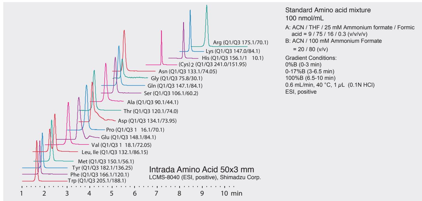
Imtakt has developed a novel column for the analysis of amino acids with LC-MS systems. The Intrada Amino Acid column achieves high-throughput analysis without tedious pre- or post-labeling methods. Optimization of analytical run times and resolution is accomplished by varying column dimensions. Separation of leucine and isoleucine isomers, GABA isomers, and dipeptide analysis is now possible without derivatization.
