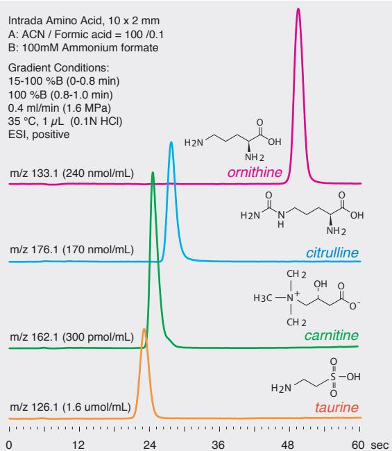
Above: One minute ultra high-throughput analysis can successfully be performed on a 10mm length column.
