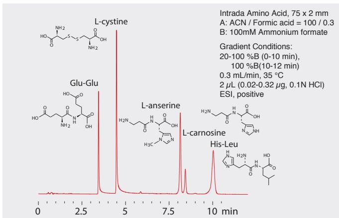
Intrad Amino Acid is an excellent choice for the analysis of polar dipeptides, which are notoriously difficult to retain and separate in conventional HPLC.
