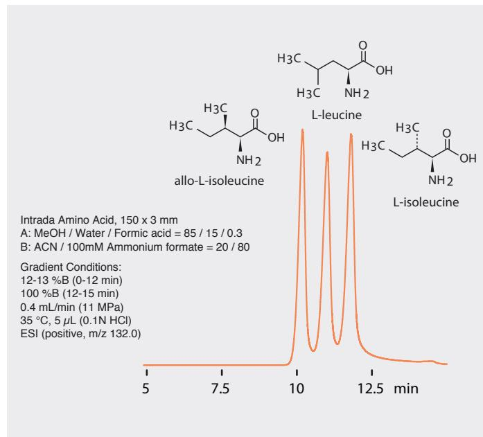
Intrada Amino Acid columns separate amino acid isomers quickly by using an optimized column length, as in the example of aminobutyric acid isomers (103Da) and leucine isomers (131Da) using 100-150mm length columns.
