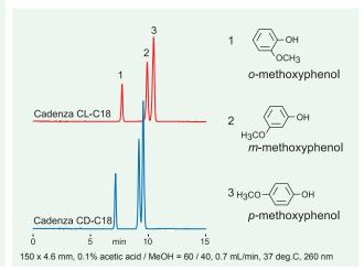
Due to its partial endcapping, the Cadenza CL-C18 opens a new world of separation possibilities. Almost all recent ODS columns have complete endcapping. However, complete endcapping makes some separations impossible. Conversely, ODS columns without any endcapping provide poor elution characteristics due to the influence of silanol. Our new Cadenza CL-C18 with partial encapping uniquely optimizes the remaining silanol.
