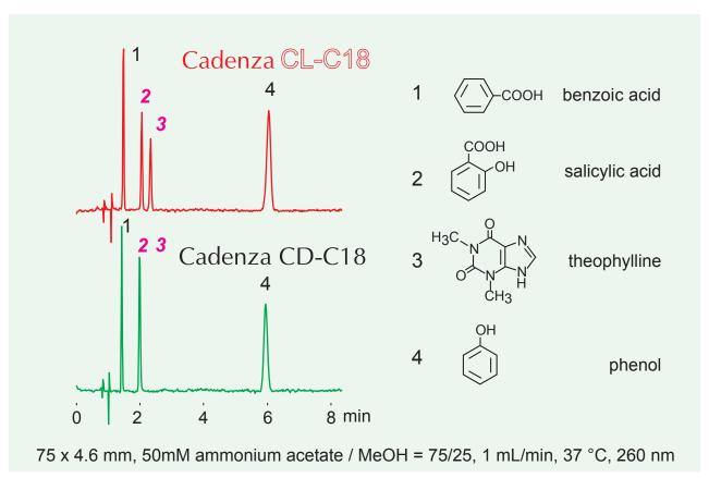
Cadenza CD-C18 and Cadenza CL-C18 have the same base silica and ODS ligand density. The only difference between the two phases is the amount of residual silanols on the silica surface.
