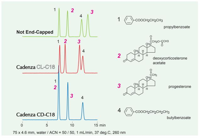
When molecular structures contain oxygen-rich functional groups, different selectivity can be obtained on different ODS phases. The neutral compounds with oxygen-rich structures had improved separation on CL-C18 due to the effect of silanol.
