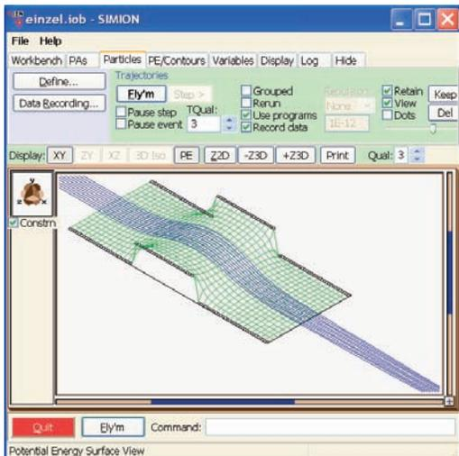
**Viewing of the system is highly interactive,** allowing adjustment of parameters and viewing of the system even during particle flight (trajectory calculation). SIMION supports cutting away volumes to see trajectories inside, zooming, viewing potential energy surfaces, contour lines, and trajectories, and reflying particles as dots for movie effects.
